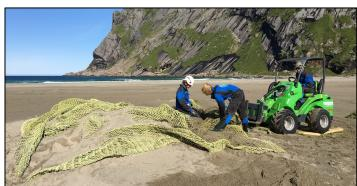
Figure 13: Preventing the wheel loader from getting stuck during operations required fishing net mats to reduce spinning of the wheels (bottom), and most often also wooden planks beneath the wheels (top) to spread the machine's weight and provide a solid surface to drive on. This was increasingly important as the sand around the item being dislodged became disturbed, and to allow the wheel loader to get close enough to the edge of the mound.
