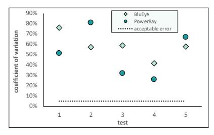
Figure 2: The coefficient of variation (i.e., the standard deviation divided by the mean, expressed as per cent) of the estimated field of view calculated from different still images of each test video (pass over transect). Results are shown for both drones. The stippled line shows what is typically the maximum variation allowed in scientific work.
