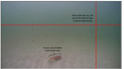
Figure 1: Sample still image from ROV videos showing one of the bottles on the rope transect used to set the scale (i.e. pixels per cm), and subsequently to determine the field of view (area shown in the image, calculated as width x height and given in m<sup>2</sup>.
