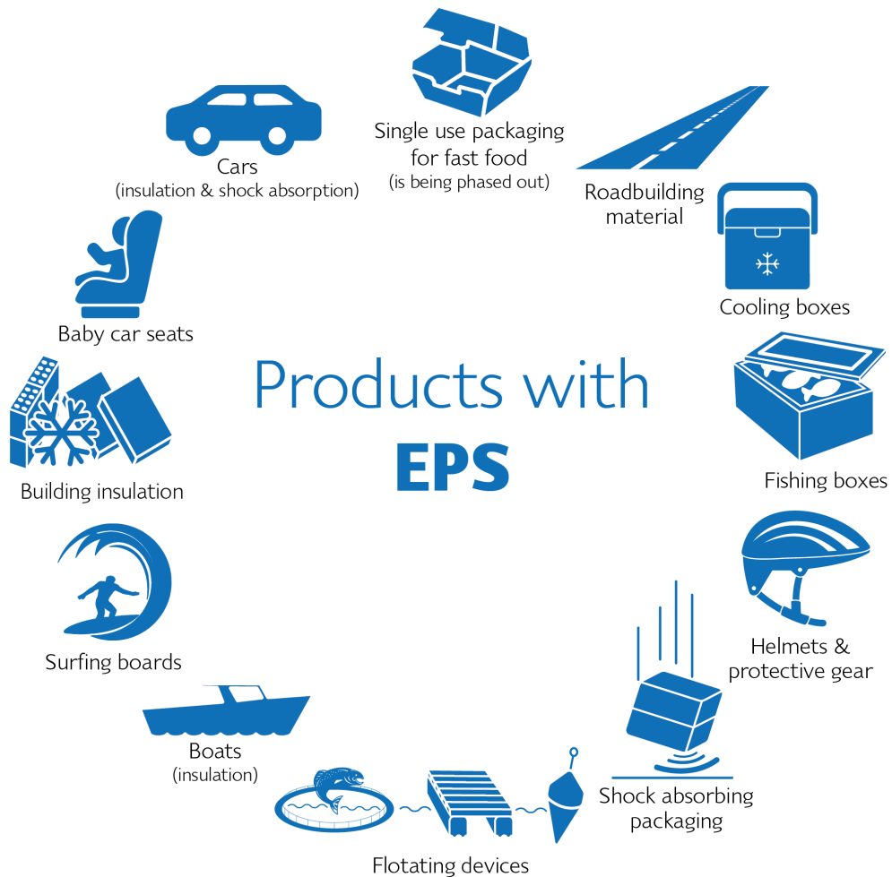
Figure 5.1 Products and materials that contain EPS or other types of expanded plastic.
