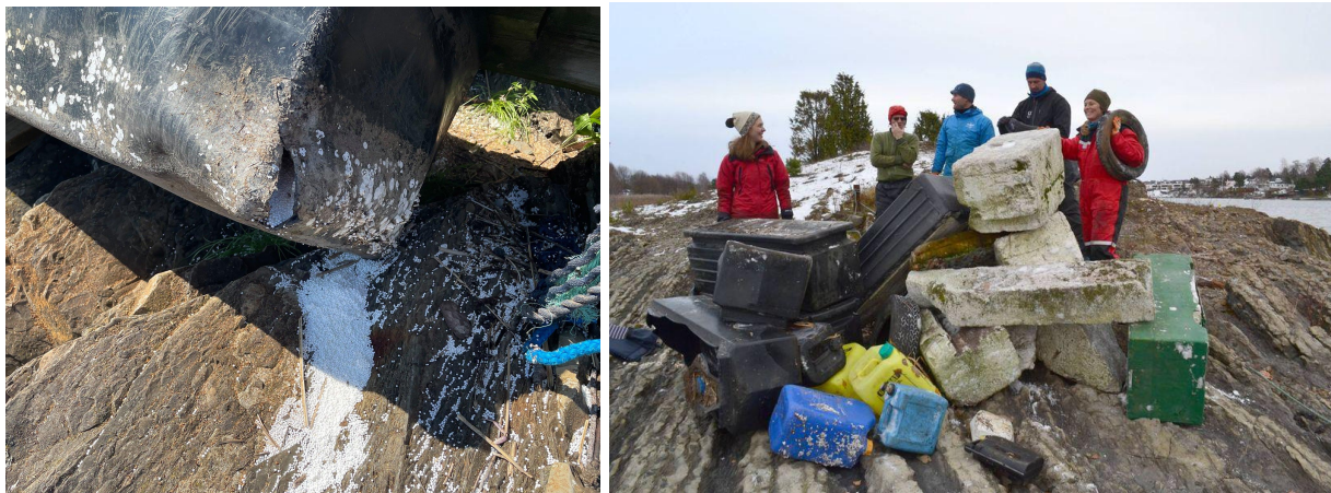
Figure 3.11: Left: EPS leaking out of a covered pontoon. Photo: Oslofjorden friluftsråd. Figure 3.4. Right: Damaged floating elements picked during beach cleaning. Photo: Oslofjorden friluftsråd.
