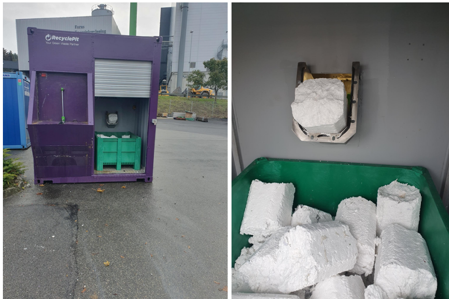
Figure 4.3: EPS-compressor and pressed bars of EPS.
