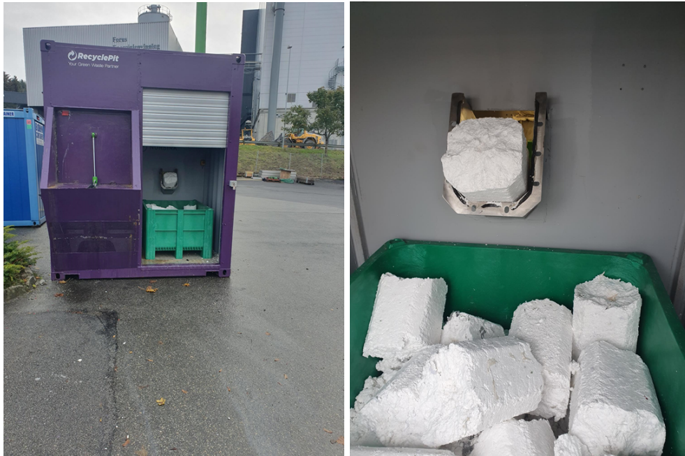
Figure 4.12: EPS compactor and EPS-bars after compression.
